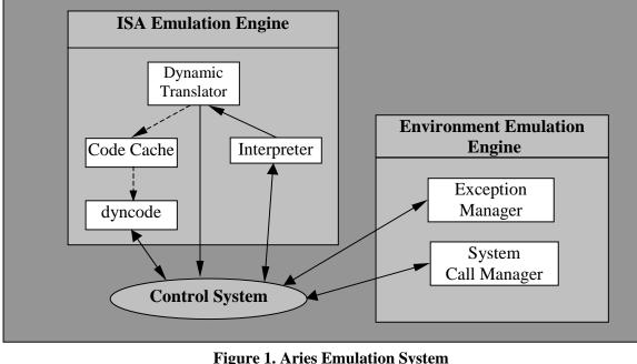
Figure 1. Aries Emulation System → Data Flow → Control Flow
