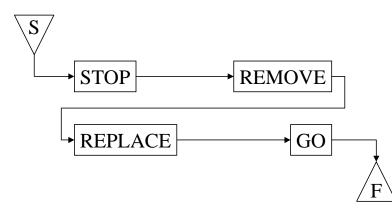
of dependency is correctly assigned. Considering the need to change a flat tire provides a simple example. The diagram indicates a start point, usually by a triangle identified with an "S", followed by the activities: (1) stop the vehicle. (2)
