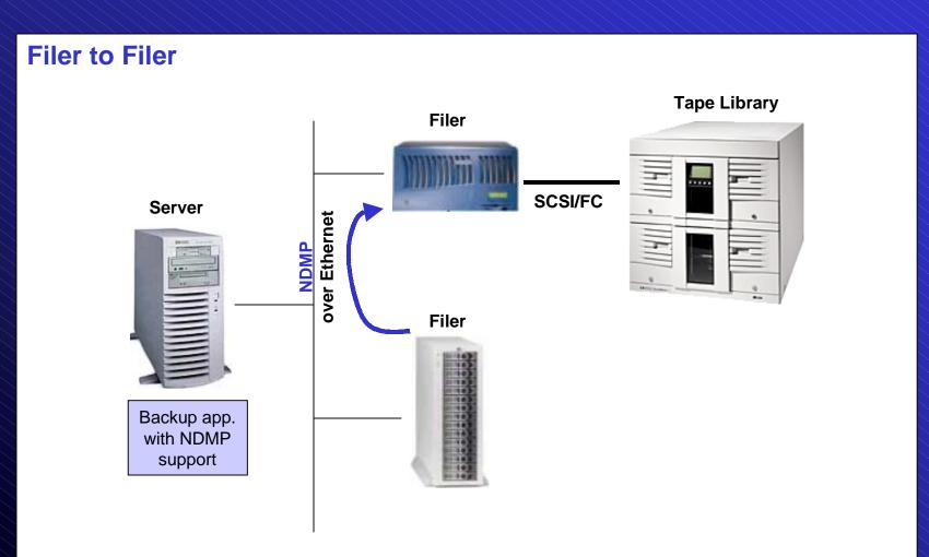
Removes backup loading from single filer using **snapshots** and **snap-mirror** technology
