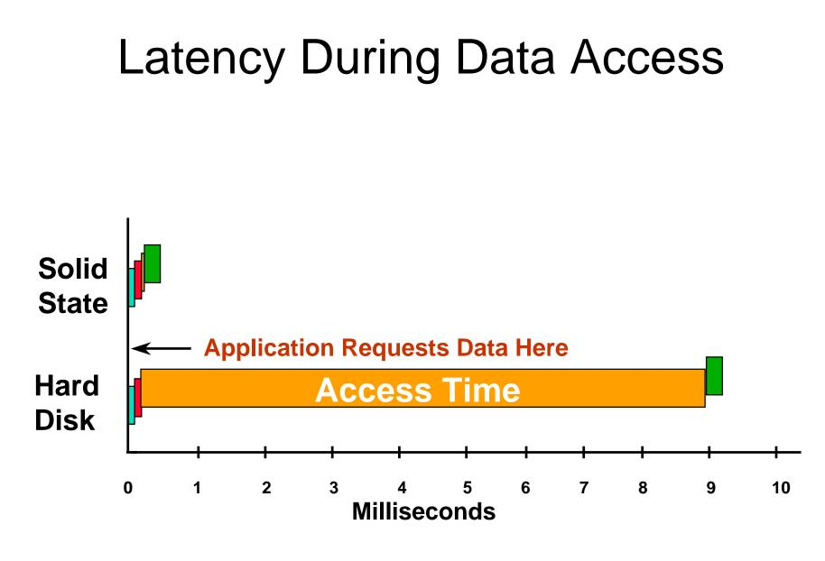
**CPU** overhead **Controller** overhead **Access** Time **Data** time
