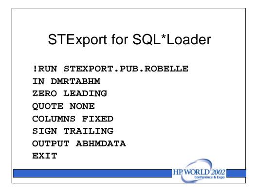
If you used Suprtool to extract a dataset into a file, you can use Suprtool's STExport to prepare the data in a format that the SQL\*Loader will accept. STExport lets him define the format of numeric data, including leading zeros and the position of the sign.
