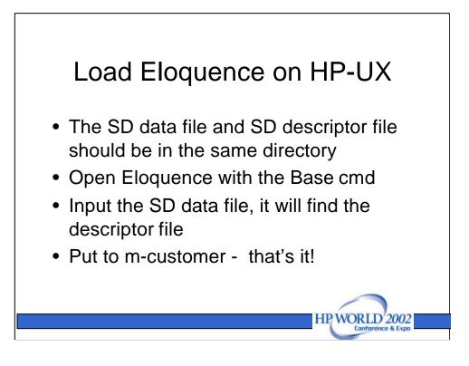
On HP-UX, inport the self-describing file into Eloquence using Suprtool:
