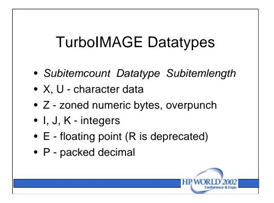
A typical data item definition is J2, where J is the Datatype and 2 is the SubItemLength, or 5X8 where 5 is the Subitemcount and 8 is the SubitemLength. The type designators are E, I, J, K, P, R, U, X, and Z.
