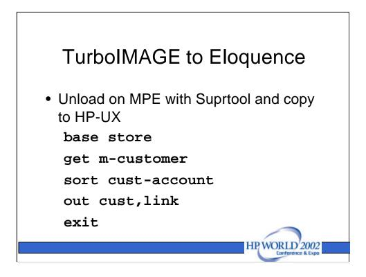
To migrate data without any conversion issues, use Suprtool. This is different from most migrations, because we do **not** need to convert the data to character format. We can transfer in the original native BINARY formats, since MPE and HP-UX use exactly the same data formats and you can have Suprtool on both servers.
