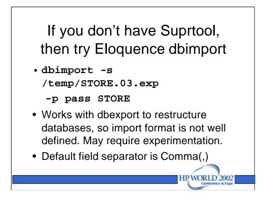
Because the Eloquence dbimport was written to go with the dbexport program and to facilitate data restructuring, files to be imported must have a name in this format:
