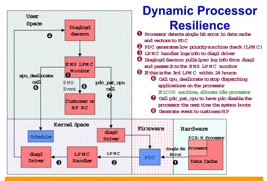
DPR makes the system fully resilient to CPU cache errors which is one of the greatest contributors to system downtime. Cache errors contribute 80% of total CPU hardware errors.
