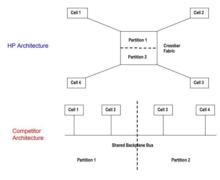
On the HP system, the crossbar logically separates the two physical partitions to provide performance and isolation.
