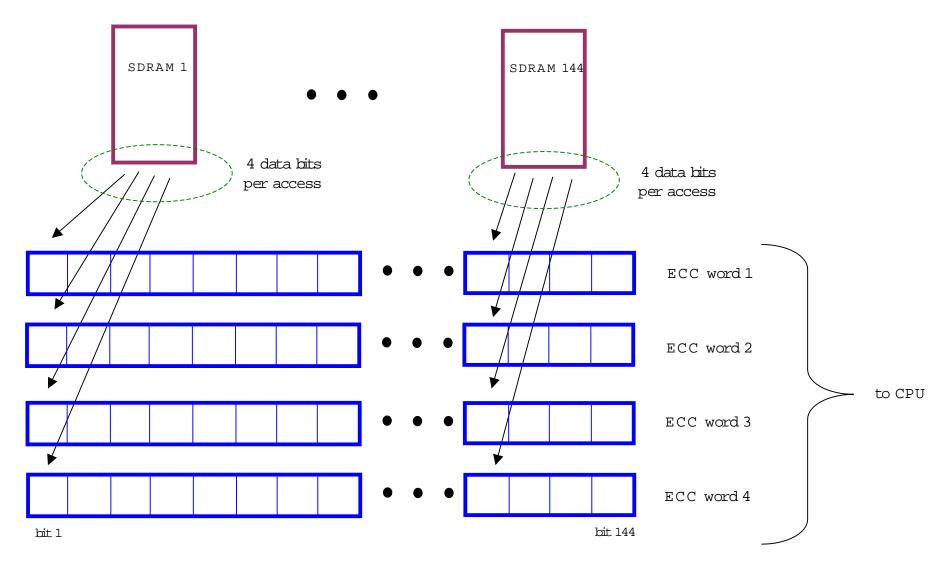
Note: no SDRAM contributes more than one bit to each ECC word. Therefore, memory system is 'redundant'
