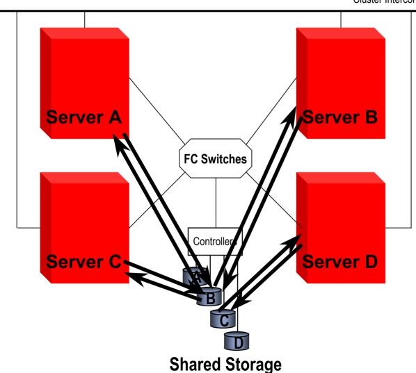
Direct Access I/O means all nodes in the cluster can talk directly to all disks in the cluster
