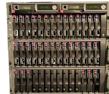
Modular SAN Array 1000 Departmental/Data Center
