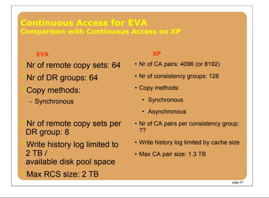
XP: Consistency Groups only used for async (which is used for > 10km)
