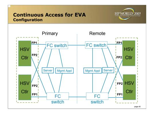
2 SANAppliances, being 1 per site. Advised is to have the SWMA on the primary site shutdown and manage everything from the SWMA on the remote site. On the SWMA, 2 components are important: HSV Element Manager and DRM-UI. The SWMA must be able to 'see' both the Source and Destination Storage System.
