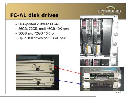
SCSI drives only have one port, because of the number of signals/pins required for the interface, with no redundancy or load balancing option of a second port. FC drives have two ports, providing redundancy and load balancing.
