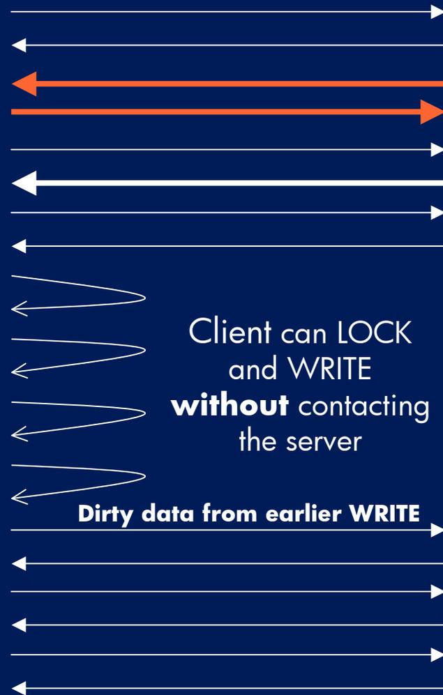
Client can LOCK and WRITE **without** contacting the server
