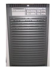
4 cells, 16 cpu's 64 DIMM slots 32 PCI slots, 17U high, 19" rack
