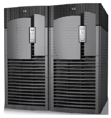
16 cells, 64 cpu's 512 DIMM slots 192 PCI slots
