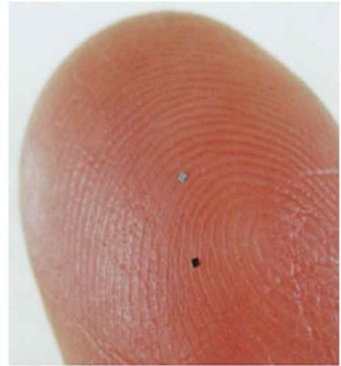
The Meu-chip is built using a conventional CMOS process.
