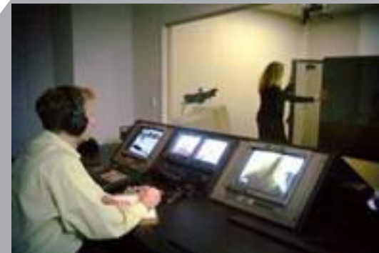
Audio and video equipment, and one-way mirrors, to observe how products are used
