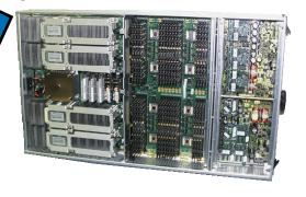
Superdome "Pinnacles" cell board for PA 8800, 8900, and all Itanium® processors
