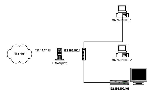
The two PCs and the HP 715 are connected to the IP Masq box via a simple hub (the "hub" can be anything from an inexpensive hub to a large, managed switch). The IP Masq box is connected to "The Net" by any one of a variety of options from dial-up 56K to xDSL or cable modem.
