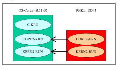
This diagram also shows that while the patch files will be delivered in a fileset that shares the name of its ancestor, every fileset in a product does not need to be found in one patch. Several patches may exist for the same ancestor fileset, but there are restrictions against the delivery of the same file in unrelated patches.
